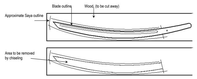
When removing the wood from the inside of the saya, one must follow (for the most part) the blade geometry.
