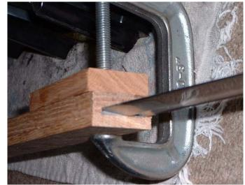
unclamped to see if the blade can slide out relatively easily. It shouldn't come out too easily, but it shouldn't be forced. It shouldn't slide out on it's own, and probably not even by shaking it. It should slide out without cutting through a towel while holding the blade.
