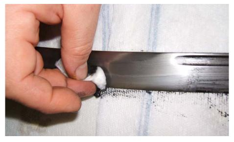
of baking soda to neutralize any residual FeCl that may be left on it. Finally, coat the blade with a fine layer of mineral oil.
