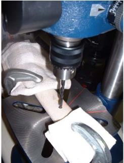
Once the main hole is drilled through the steel, I remove the blade from the drill press and clean up the area on the nakago around the new mekugi-ana with 320 and then 600 sandpaper and oil.
