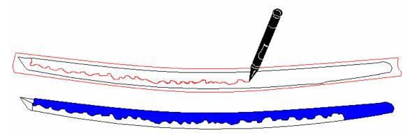
Now, you can either carefully cut it with an exacto blade, making sure you don't push hard enough to scratch the steel, or you can do this by outlining the blade, removing the tape, placing it on a glass or similar surface, and replacing the tape. I cut it on the blade, taking care to not push too hard. Work it off slowly, and trim it if necessary more then. The tiny scratch that may get put on the blade will be polished off anyway... just be careful.
