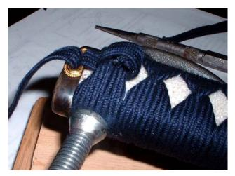
When you get to this point, you must carefully tighten the knot by working the end of the ito all the way around so that is underneath the folds. Very fine needle nose pliers are good for this. Reach inside carefully, and rotate the knot, tightening it. If you have too much ito, pull it out carefully, and trim it again.
