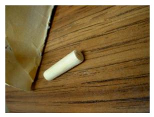
Mekugi fit should be tight, but not too tight to insert it by tapping gently with a very small hammer or small block of wood. The picture below shows about where mine get too tight to push in easily with a finger.
