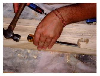
Start chiseling from the center, and take the wood out of the deepest part first. Work the wood out as smoothly as possible to the end, and then work back the other way. If there is a grain to the wood that isn't straight, chisel against a descending grain like in the following graphic.
