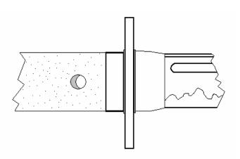
The mekugi-ana is not lined up with the nakago, and the steel overlaps slightly at the rear of the mekugi-ana. This is good. This is adjusted by removing the tsuka, Taking off the fuchi, and sanding off *almost* the amount of the overlap. It should be pushed on reasonably hard as to not allow any movement of the other components.
