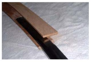
resin that would show me the shape of the piece that needed to be cut to fit inside the first tsuka half, I determined that a better quality filler than what I was using would suffice for the wood that would have to be left on. The technique ended up fitting more accurately, was stronger than wood, and impervious to oils and water.
