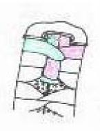
When finished, your knot should look something like the one in the picture to the right. Once your rice paste or glue dries, you can adjust the ito where it runs through the shitodome so that it's centered, or it occupies the entire space. In order to do that, you may have to insert a thin tool to move the ito over. Don't pull too tightly or push it so hard with a tool that you fray the silk!
