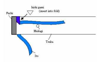
Then, after the hishigami is inserted in the first fold, the fold is continued on over and another hishigami is inserted into the new fold, under the ito.
