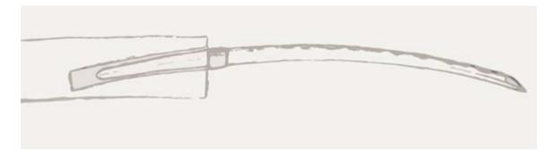
Once you know what the general curvature and length is for the tsuka, trace the dimensions to a piece of wood you will use to make it. I make two every time. Making two has saved me many times when I went back to the one still on the wood that hasn't been cut yet to re-confirm dimensions when final shaping of the tsuka.
