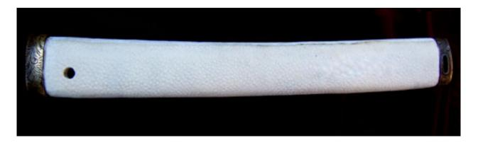
The fuchi and kashira are fit by measuring the space they would take up on each end, mark it with a pencil, and hand sand or file the ends to the appropriate size. I measured the progress many times, and despite that, still manage occasionally to sand too much off. Sand or file less than you think. That seems to be a rule.
