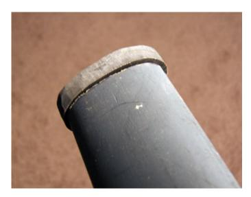
When I fit an iron koijiri to a saya, the koijiri must be fit, then the saya must be finished, such as lacquered, and then when the saya is done, the koijiri needs to be put on. This means the space the finish takes up must be accounted for prior to fitting the koijiri.
