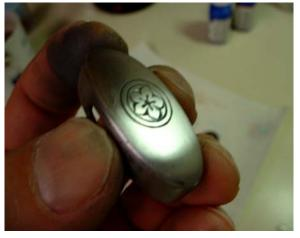
I then treated the polished parts with selenium dioxide for 30 seconds at a time to make them "Blue." In case you're thinking, "That chemical sounds familiar..." It probably does. It's the active ingredient in gun bluing.
