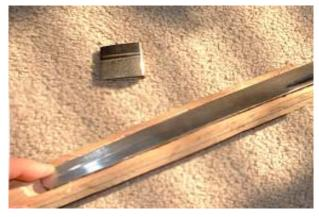
To determine where I needed to sand, I use a variation on a technique used to gauge variances in a level surface when machining automotive parts. For this I used carbon paper. If you don't have it, you could just rub the tang with a soft-lead pencil or art charcoal first.
