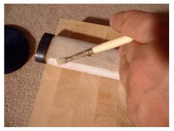
The strips are glued using boiled Japanese rice mashed into a paste (with a little water added). This glue can be made easier by mixing Elmer's glue with a touch of water.
