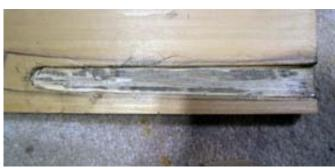
Once I get a good rub, I use a jig and sand the opening smooth. Test fit the sword and work with fine sandpaper until you get a good fit.
