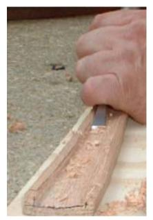
Considering chiseling, above all make sure they are sharp. Take the time to learn how to sharpen them... it pays big dividends later. When removing wood, I use a wide chisel to get the bulk of the tsuka hollowed out. I also shape the chisel so it's the same width as the shinoge-ji. If your chisel isn't, it will save you heartache later to grind the width of the chisel to the same width as the shinoge-ji.
