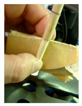
To sand the mekugi, I chuck the bamboo in my drill press, and at a marginally slow speed, run the drill while holding a sanding block with 220 paper on it against the bamboo. You must measure often, like every ten or twenty seconds of sanding. It's important to leave it both longer and bigger in diameter than the hole size by a wide margin because when checking, you will almost always find that you'll have to sand it some more to smooth it or straighten it.
