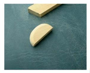
Traditionally, the kurigata is either dove-tailed and fit to the saya, or put in like a mortise joint. I install mine with a set pin, and glue it so it's strong and won't come loose.
