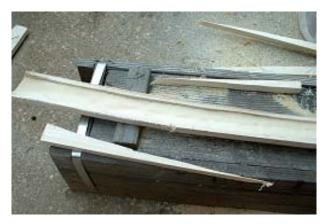
After sanding the saya, Leave about  $\frac{1}{4}$  inch (6 mm) of space on either side of the blade. I'm not really sure if there's a specific amount that should be left, although it will depend on the width of the blade. It appeared to me that my other saya were about  $\frac{3}{16}$  inch (5 mm) here, so that's what I left. The next thing I do is to place the saya on the second half and mark where it should be cut to match the first one.
