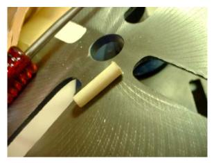
I feel that it's worth making another one if I have a poor fit--this retainer is important! Once the diameter of the mekugi is proper, I insert it and mark where I want to cut it down to. I always leave some excess on either end, as the mekugi edges should be nicely rounded off on each end. Hand sand the ends, and be careful!
