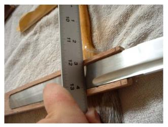
Using a straight edge assures that the nakago sits deep enough in the tsuka. There should be NO space between the straight edge and edges of the tsuka. NOTE: For forming the cap for the tsuka, it will be extremely helpful to have the shinoge-suji level with the edges of the tsuka.
