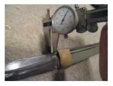
I measure the tang in a dozen places, and transpose those measurements to the inside of the tsuka. I then draw the lines onto the tsuka from the nakago. Consider the angle of the shinoge-ji and ji, and take care to sand the tsuka accurately.
