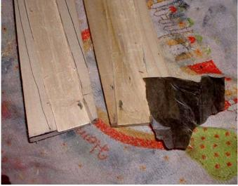
When I get to the finish sanding of the saya halves, I start fitting the habaki. In order not to cut too much off, I put the two sides together over the blade, and wrap carbon paper around the habaki, and slide it in until it strikes the wood. The mark where the habaki strikes the inside of the saya when the blade is slid in is where I carefully chisel away until the blade and habaki fit correctly.
