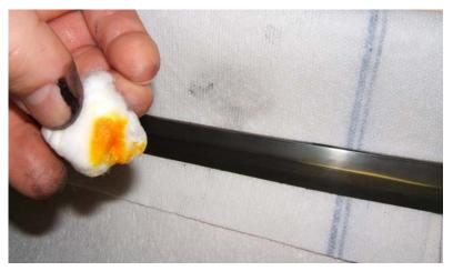
the blade very well with lots of fresh water, and dry it off. Don't neutralize it yet. Turn it over and make sure that none of the FeCl solution ran to the other side and marred it. If so, polish it out. It has to be even to look nice.
