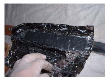
If too much is put in, it will compress the tang and the nakago will not slide in when it's dry, or you may split the wood, or at the least, the "cap" won't fit on, and you'll have a mess from Hell trying to clean it all out and start all over. On the other hand, enough must be used or the result will be voids in the mix, and that means a weak substrate. I carefully level out what I put in with a straight piece of wood.
