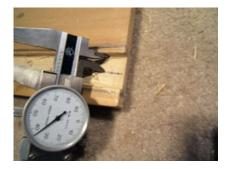
You'll have to retry the fit very frequently, twice as frequently as you think you should. Move greater amounts of wood with a sharpened chisel by hand.
